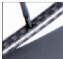
Sapim bladed spokes with hidden nipples for additional aerodynamics
