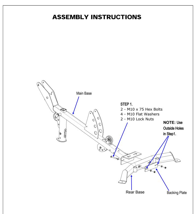
Step 1: Attach Rear Base to Main Base and Backing Plate using outside holes. **Only finger tighten now.**
