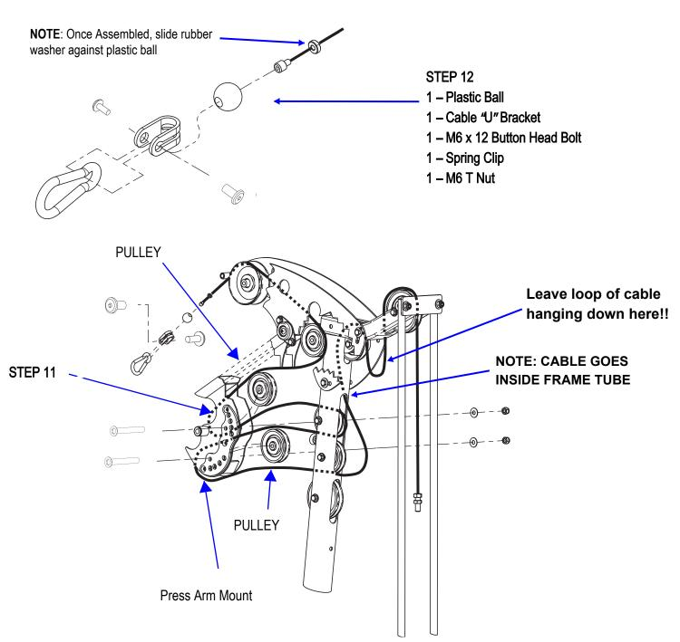
Step 11: Attach Upper Cable. Begin by running Upper Cable from back of machine to front as shown. Weave cable through pulleys and out over the Wide Groove pulley.
