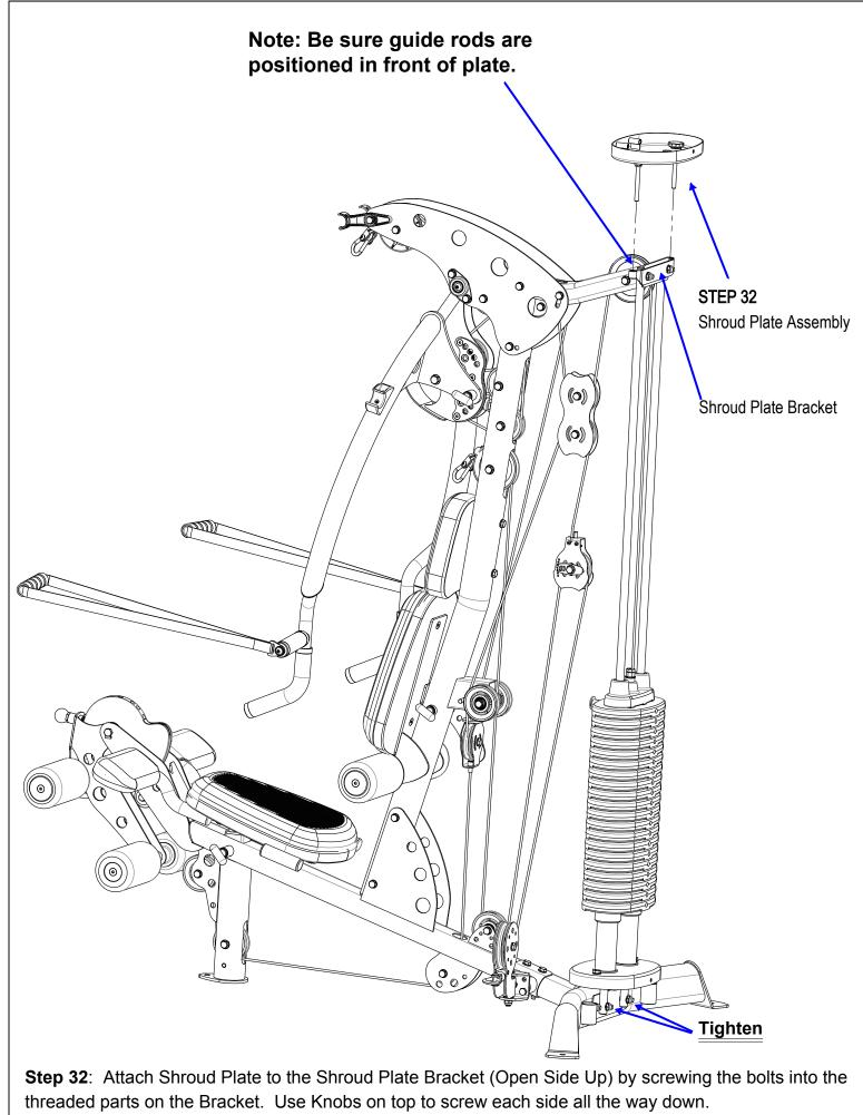
Tighten Main Upright bolts Now. Tighten bottom bolts of Guide Rods Now.
