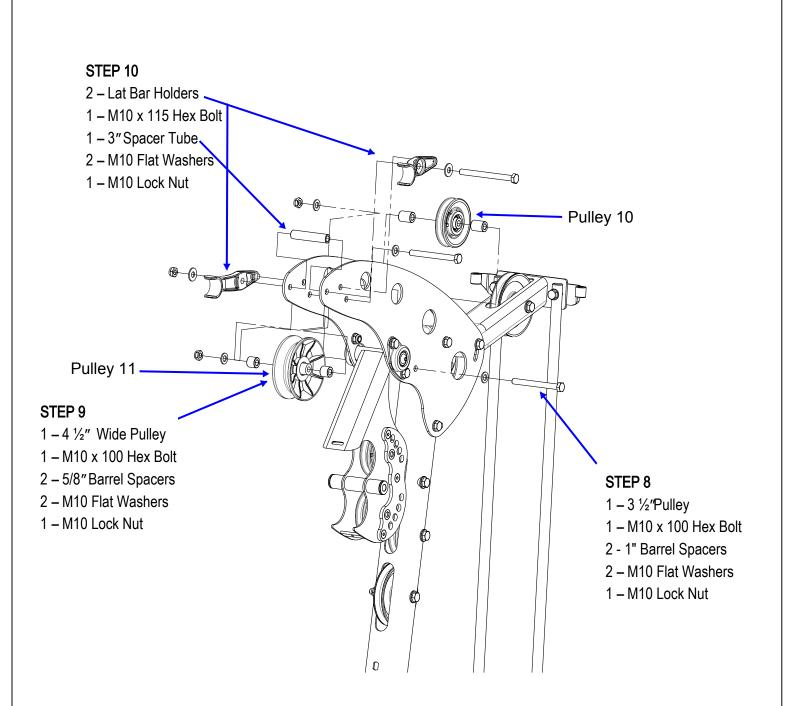
Step 8: Attach Pulley 10 to Top Beam Plates (just behind bearings) with M10 x 100 bolt.
