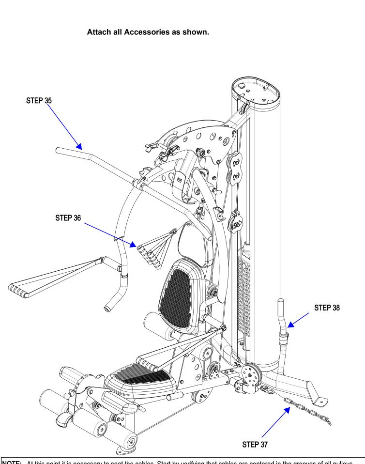
**<u>NOTE</u>**: At this point it is necessary to seat the cables. Start by verifying that cables are centered in the grooves of all pulleys. Next, select a weight you can comfortably handle on the bench press. Perform a seated bench press and hold the first repetition at arms length. Now, lightly bounce the weight up and down for about 5 seconds. This will seat the cables into the pulleys. You may readjust the cable stops at this point if needed.
